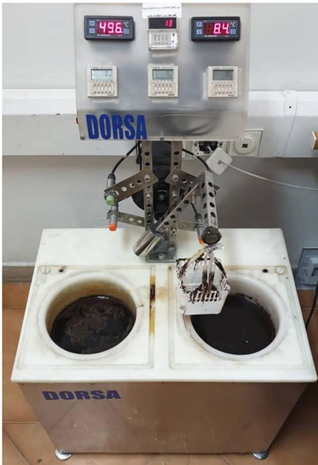
**Fig. 3** Coffee thermal cycling of the specimens with 5000 cycles
