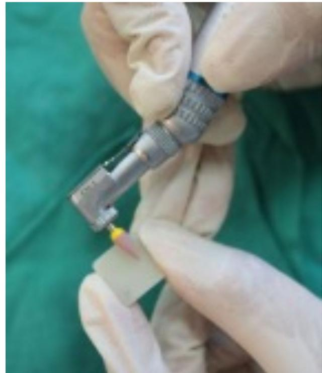
**Fig. 2** Pre-polishing of the specimens with W16Dmf
